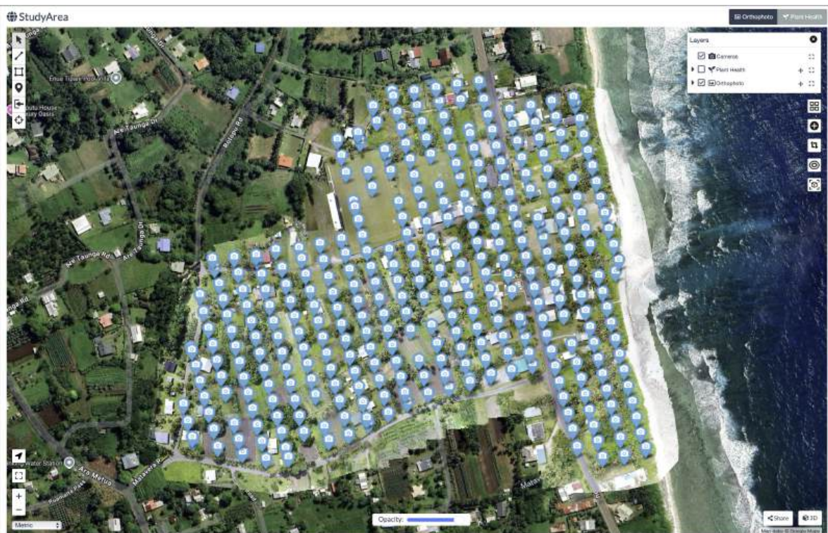
Figure 1: Positions of 347 RGB aerial images. Source: Asian Development Bank visualization using OpenDroneMap 3.6.0 (2025).
