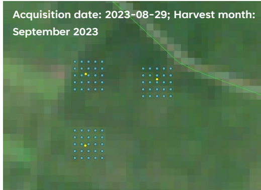
Figure 3. Example of 5 x 5 pixel window creation
