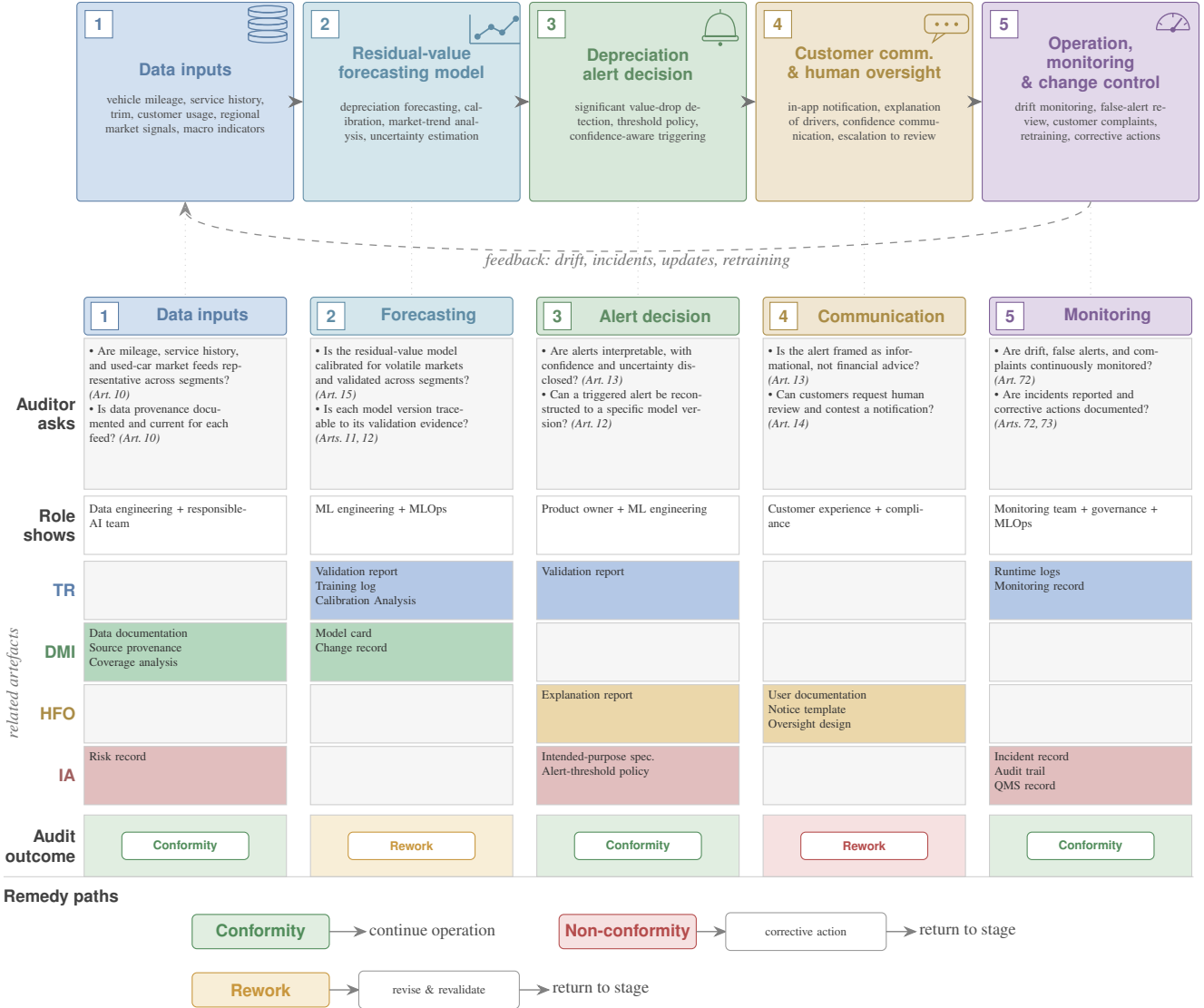
Figure 3: Evidence-centric system-level QMS view for the automotive residual-value agent. For representational clarity and space reasons, the figure condenses the seven-stage lifecycle in Figure 2 into a five-stage operational pipeline. It maps these stages to auditor questions, responsible roles, case-specific evidence artefacts, and illustrative audit outcomes, showing how quality claims, context-specific evidence, organisational responsibility, review, and corrective action can be connected for a specific AI system within a QMS. It uses the same governance clusters as Figure 2: technical robustness and reliability (TR), data and model integrity (DMI), human-facing intelligibility and oversight (HFO), and institutional accountability and governance (IA). The feedback and remedy paths illustrate how drift, incidents, rework, and non-conformity can challenge existing quality claims and trigger review, revision, corrective action, or revalidation. The specific artefacts, evaluation methods, review procedures, and evidence thresholds remain system- and context-dependent and must be determined according to the system’s intended purpose, risks, affected stakeholders, and deployment conditions.
